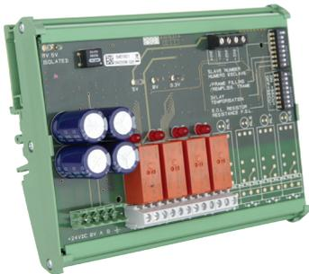
Programmable 4 or 8--relay module can be located closer to the actuators for cost savings.
