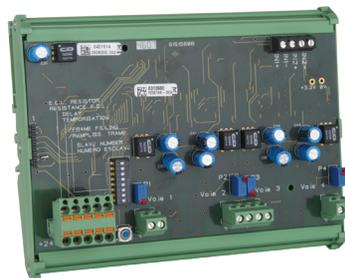
Addressable 4-analog-output module that delivers four analog 4-20mA signal outputs (detector output copy, min, max, average of a group of detectors) for connection to a datalogger, a PLC, a Building Management System (BMS), etc.
